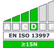
\* For dulling during cut resistance test (6.2), the coupe test results are only indicative while the TDM cut resistance test (6.3) is the reference performance result.
